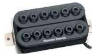
tapping control, that lets you use only a single coil in the pickup, thus generating the characteristic single-coil sound.
