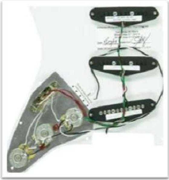
Stratocaster Pickups, Wiring and Controls
